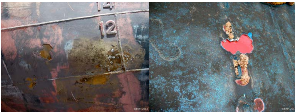
Figure 3. Biofouling and biocorrosion on ship hulls. (Photograph: Estaleiros Navais de Peniche, S.A.)
